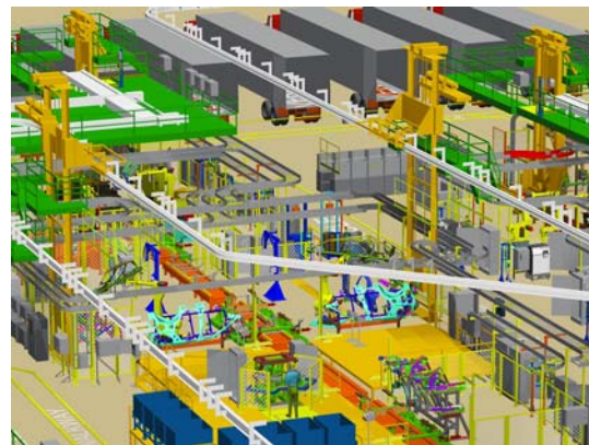
Figure 7: Establishing a 3D-factory layout by use of predefined objects (UGS)
